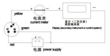
(Current output mode wiring)
