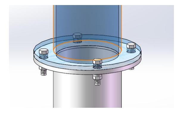
The assembly of the 1.5m upper rod and the lower rod is fixed together with four nuts and bolts. The nuts and bolts for connection are attached to the 1.2m pole when shipped
