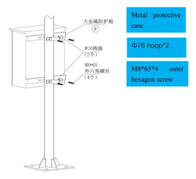
1. The square tube on the back of the protective box has been welded with the protective box before leaving the factory. When installing, just align the two hoop mounting holes with the square tube mounting holes of the protective box, and then use four 8\*65 External hexagon screws, 4  $\Phi$ 8 flat washers, and 4  $\Phi$ 8 spring washers fix the protective box on the main pole.
