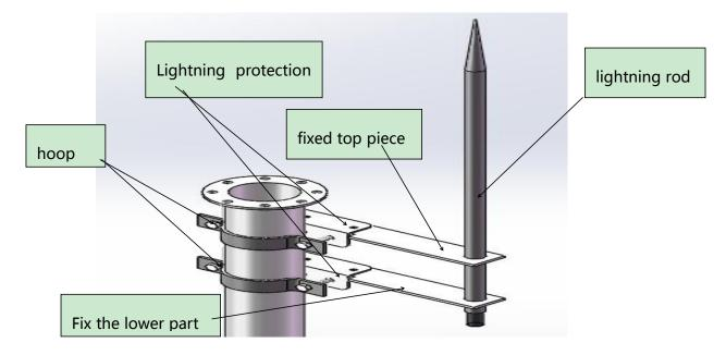
1. Pass the lightning rod through the upper fixing hole, and screw the threaded rod head of the lightning rod into the screw hole of the lower fixing piece to tighten;
