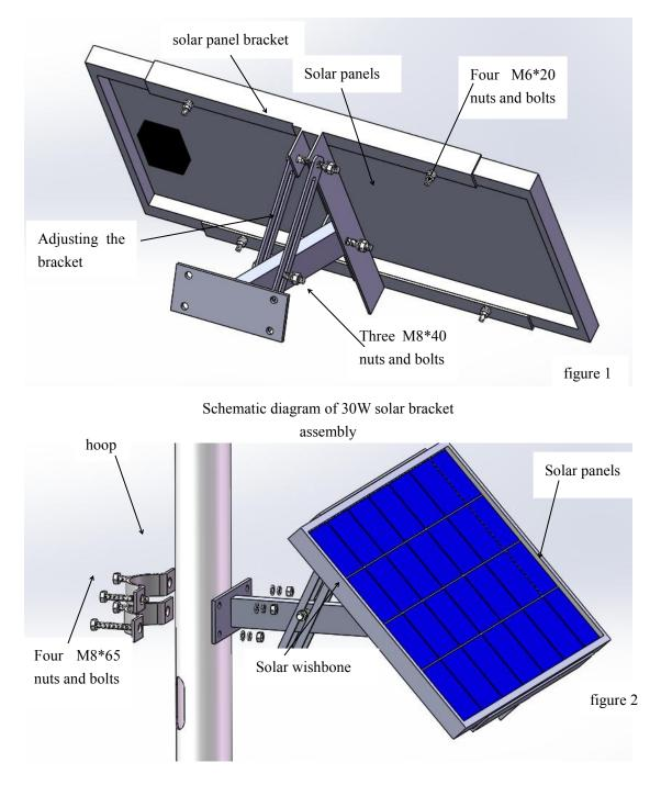
1. Before installation, please check whether the accessories are complete and whether the solar panel is damaged.
