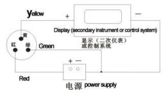
(voltage, pulse mode wiring)
