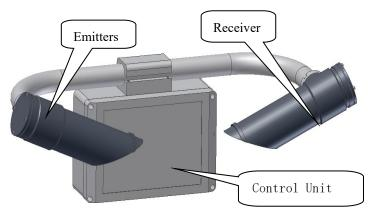
(1) Transmitter: Built-in laser tube that emits laser signals outward at a fixed angle;
