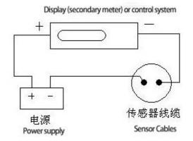
(1) If the sensor outputs other signals, the wiring sequence and function of the conventional sensor wires are shown below:
