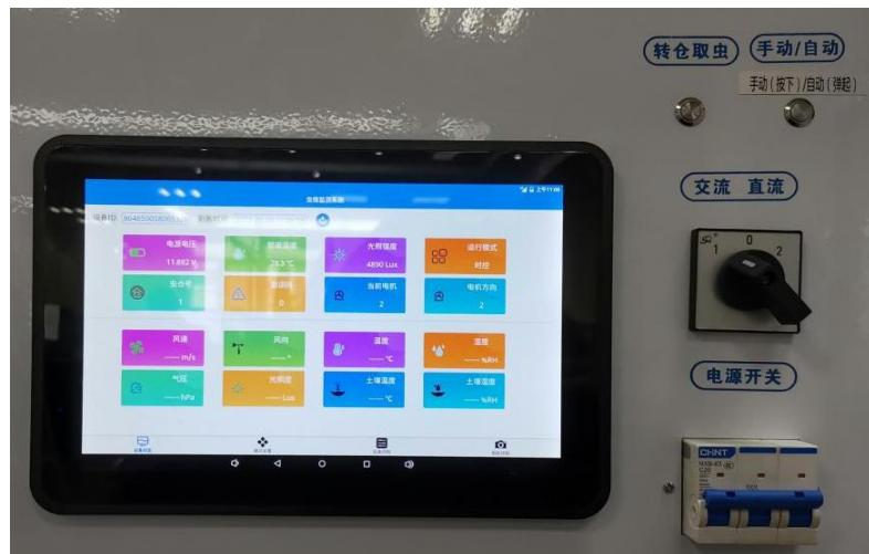
Ensure the power supply is connected, open the cabinet door of the monitoring lamp, and follow the steps on the controller panel inside the cabinet to check the operation of the monitoring lamp.
